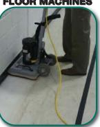
**TOMCAT'S EDGE** Series of surface preparation machines gives operators the ability to remove multiple layers of finish, without using chemicals. As we all push for new ways to increase our protection of the environment, this new approach can help achieve increased productivity and safety. Available in 20", 28" or 32".
