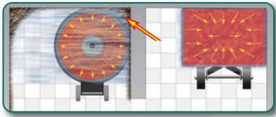
**Square vs. Round: EDGE'S** rectangular shape offers equal dwell time across pad width, unlike round pads. The square corner allows Edge to clean into corners and against baseboards better than round pads.
